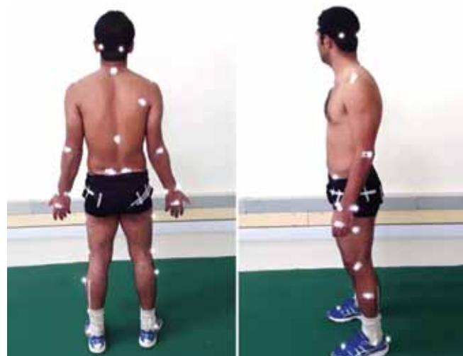
Fig. 7: Marker placement on the bowler for 3D motion capture
