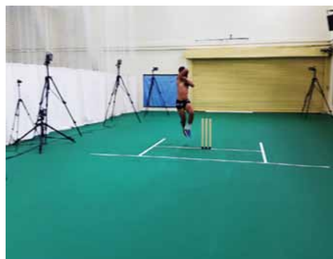
Fig. 8: Three-dimensional motion capture of the bowler in action at the lab
