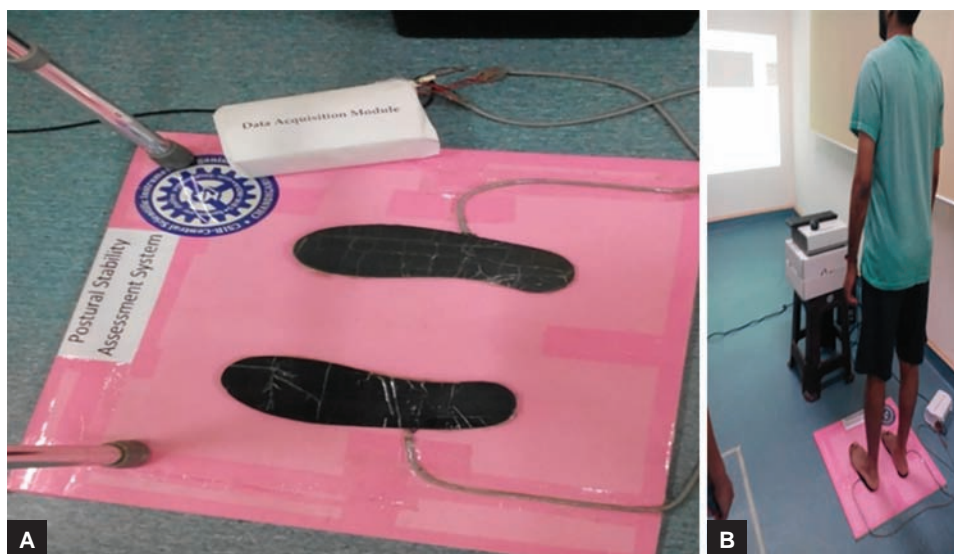
Fig. 1: (A) Image of postural stability assessment system; and (B) with subject standing on it
